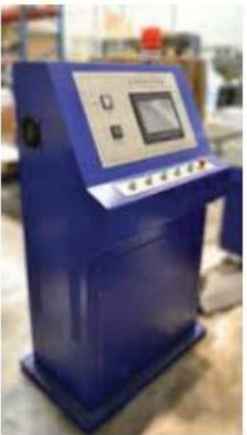
Control panel for smooth running of case maker with various premiter options for jobs with high end electrical system and servo drives - Major electrical components consists of OMRON. LS. YASAKAWA etc.
