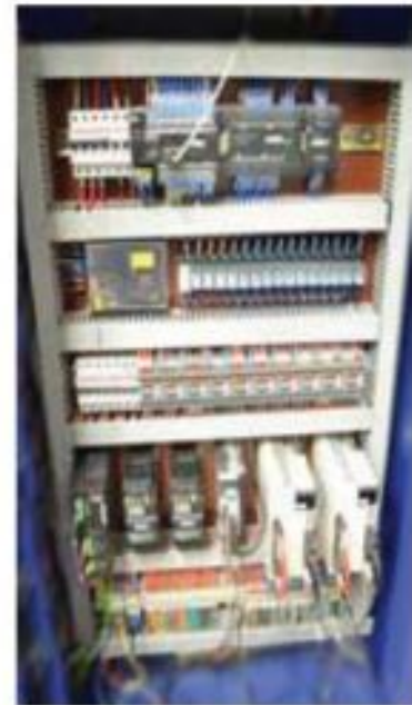
Control panel for smooth running of case maker with various premiter options for jobs with high end electrical system and servo drives - Major electrical components consists of OMRON. LS. YASAKAWA etc.
