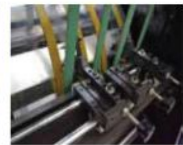
9 grooving heads with waste cleaner
