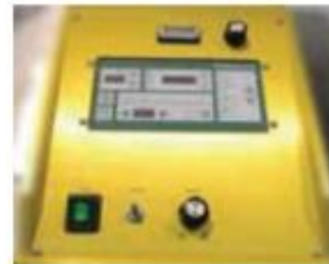
Control panel consists of counter, speed, sensor and power control
