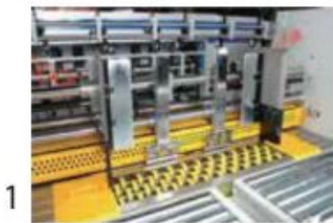
Astra Automatic Die Cutting for carton boxes with lead edge feeding ASTRA - MASTER 1670S
